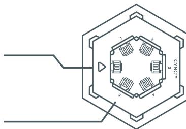
Panels are connected in series. Do not use more than one Output Port on any Hexagon Panel.
