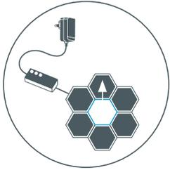
4. As with the middle Panels, after inserting the linking cable from the previous Panels, note that the panel should light up if the cable is connected correctly. If it does not light up, ensure that the control box is plugged in and turned on, and re-check your connection.
