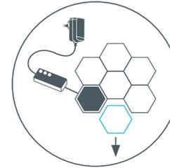
4. Remove the layout template of the Hexagon Panel you are installing. Leave the other templates in place for now.
